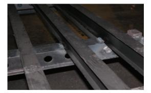
The combined strength of the Super-Sill cross members, staggered screw pattern and the solid oak flooring delivers a floor rated\* for 22,000 lbs- the best standard forklift rating in the industry. \*TTMA RP37-07
